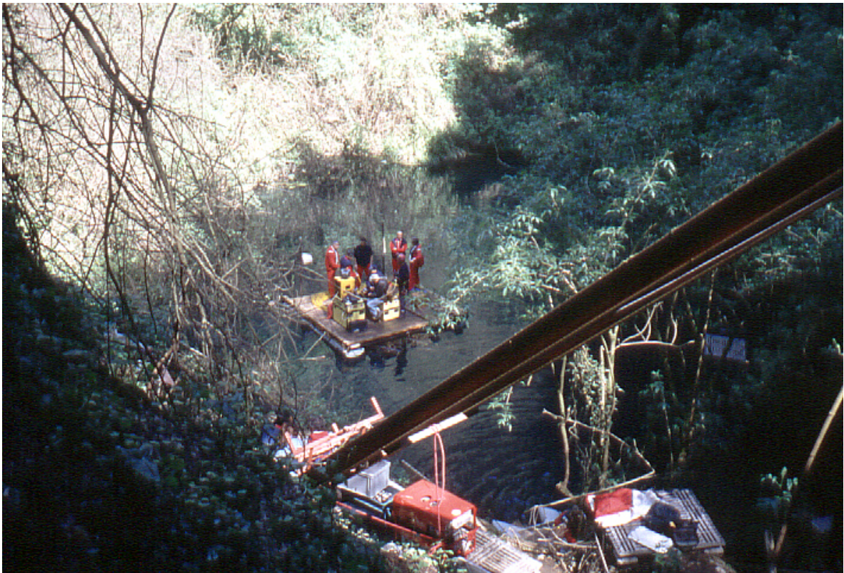
Figure 3. The ROV control floating platform at the surface of the "Pozzo del Merro"
